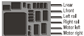
MX620 Micro processor side shown (connector pins are soldered to other side !)
