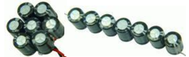
Coldcap module with 7 goldcaps (7 x 1 in series for a total of 140000uf – 17.5V)
