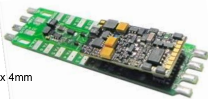
ADAPUS15 with ZIMO decoder MX645P22, 71 x 18 x 7.8mm
